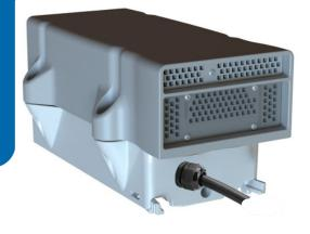
Upgrade your Sensorbee Air Pro setup with the Gas Extender Unit, compatible with both the Cellular and Modbus versions. Easily increase your monitoring capacity by connecting up to three additional gas modules, for a total of six gas sensors. Simply attach the Extender Unit to the Air Pro base with the M8 sensor extension connector. Enjoy automatic configuration and instant data transmission upon connection.
